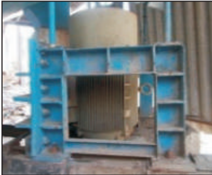
Energy Efficient Vertical Pulper Motor 150 HP
