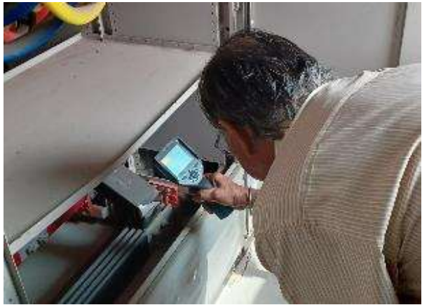
Thermal Imaging carried out by AEA at Incomer of LT PCC Panel of Ruby General Hospital
